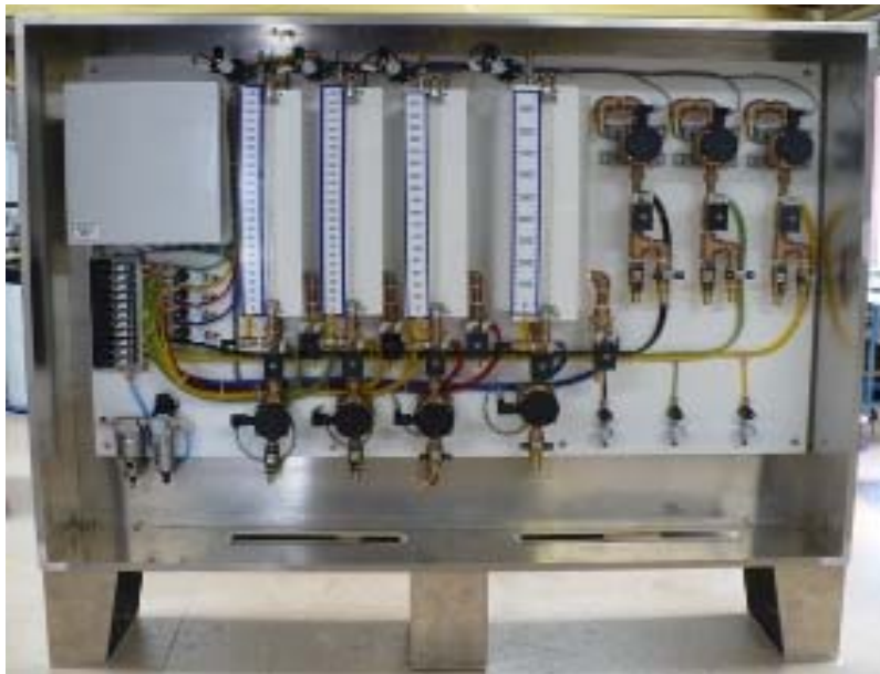
7 Unit Interface Dispenser; Units 1-4 with stainless steel tanks, units 5-7 direct feed. Mounted in aluminum enclosure
